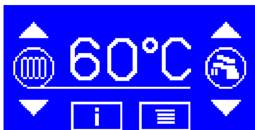
HEATING OF DHW ON
