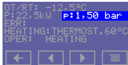
p: PRESSURE IN THE HEATING SYSTEM
