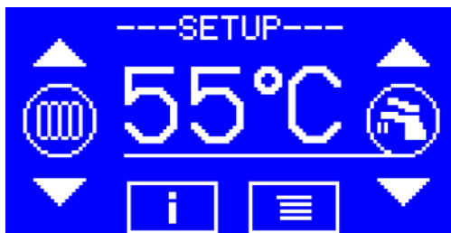
SETTING THE REQUIRED VALUE OF THE DHW TEMPERATURE
