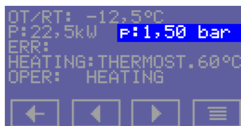
p: PRESSURE IN THE HEATING SYSTEM
