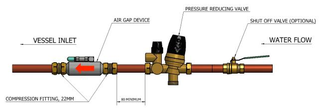
The Air Gap Device can be mounted vertically or horizontally
