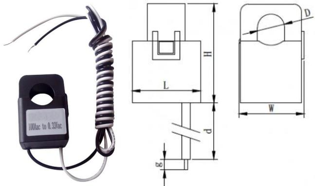
D = 16 mm (10 mm for the indirect measurement), L = 31 mm (26 mm), W = 32 mm (25 mm), H = 46 mm (40 mm), d = 3 mm
