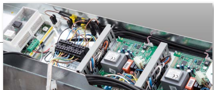
Assembly of the electronic PCBs for the management of the thermal elements and BCM
